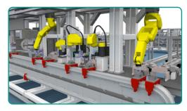
Test controls logic on new equipment in a physics-enabled virtual environment to uncover and resolve bottlenecks, safety hazards, and other challenges before startup.
